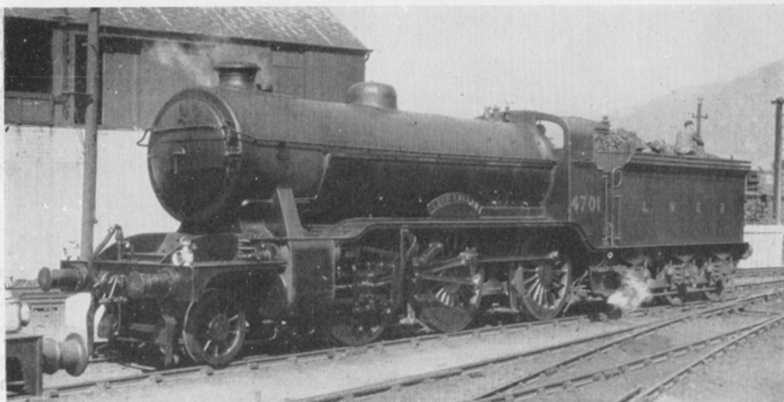
Ex G.N.R. class H 3 2-6-0 No. 4701 "Loch Laggan," as originally built (L.N.E.R. class K 2 )
